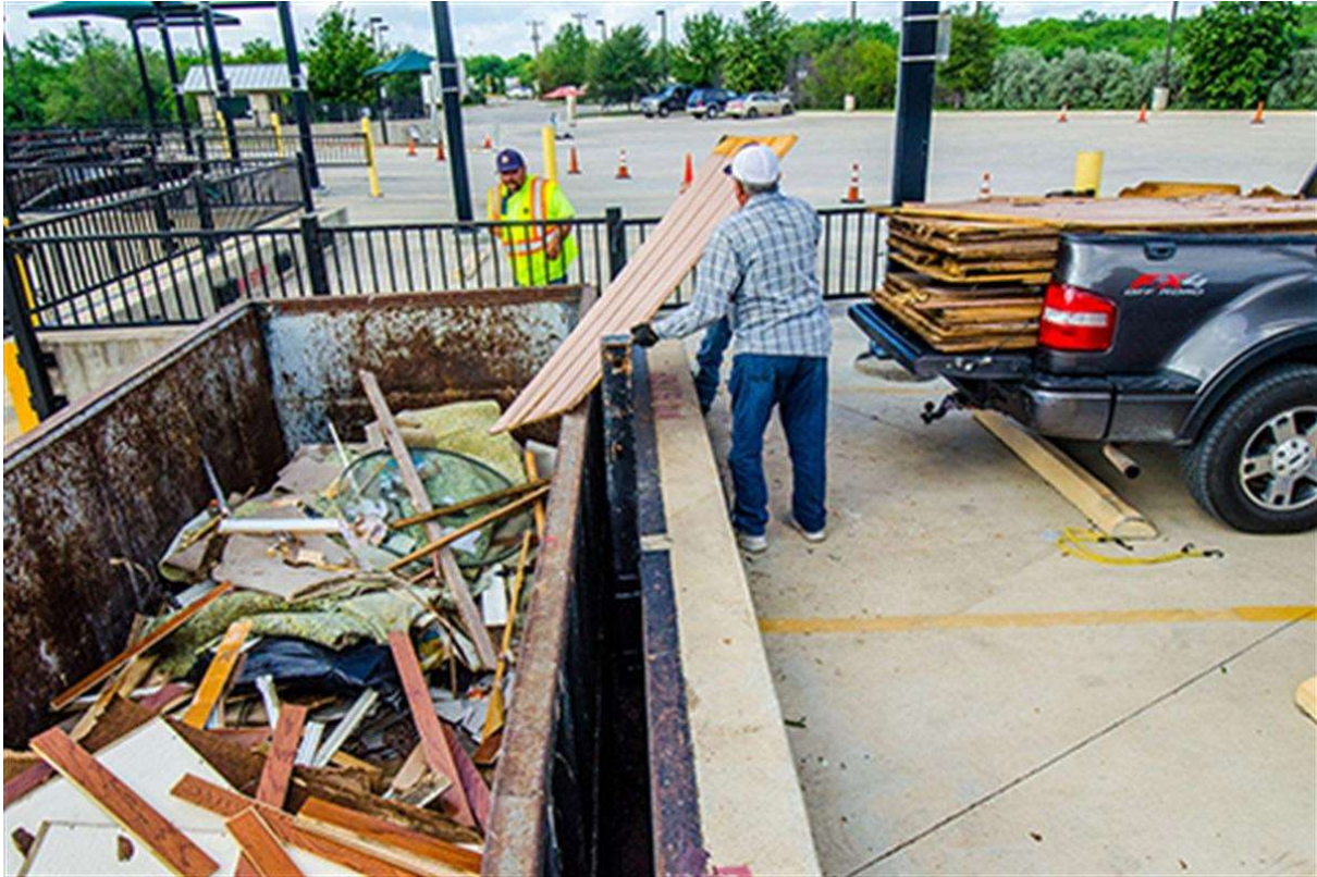
Figure 1 - Example of a below-ground direct-to-bin system
